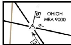
**Minimum Crossing Altitude.** The lowest altitude at certain fixes at which an aircraft must cross. Aircraft must cross the fix AT the altitude listed near the flag in the directional specified.
