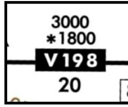
**Minimum Reception Altitude (MRA).** The lowest altitude at which an intersection can be determined from other NAVAIDs. If higher than the MEA, it is indicated with the following figure.
