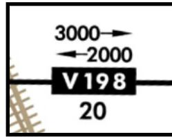
**Minimum Obstacle Clearance Altitude (MOCA).** The MOCA provides obstacle clearance for the entire airway segment but only provides adequate navigation signal within 25 statute (22 nautical) miles of a VOR. A MOCA is only shown on the Enroute Low Charts and only published when it is lower than the MEA. When shown, it is preceded by an asterisk.
